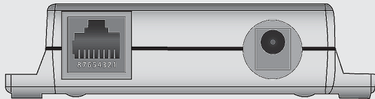
Standard RJ45 Jack Configuration- For 802.3af compliant units
